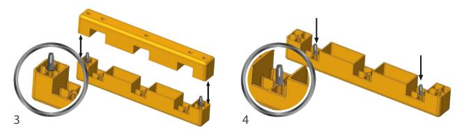
After taking apart the 2 struts from each other, remove the pins from the struts.
